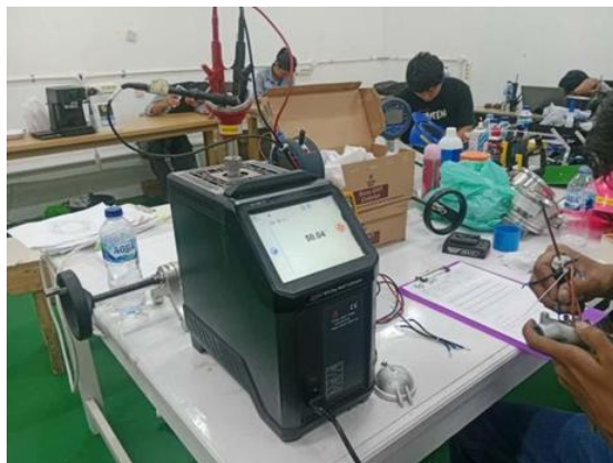
Gambar 4. Kalibrasi RTD (Resistance Temperature Detector)
