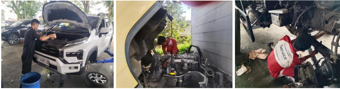
Gambar 2. Pengisian Air Radiator, Pelepasan Alternator, Serta Pemasangan Busing Per
