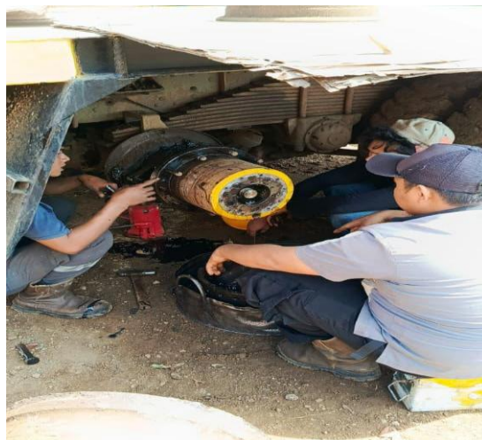
Gambar 3. Penggantian O-ring Final Drive Truck Trailer .
