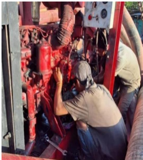
Gambar 2. Penukaran Injection Pump
