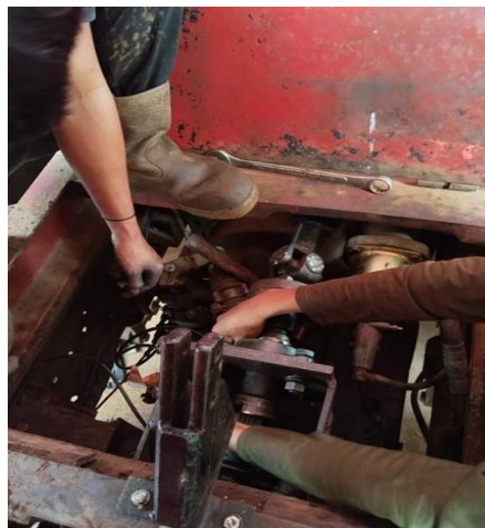
Gambar 2. Pemasangan Gear Box Power Take-Off
